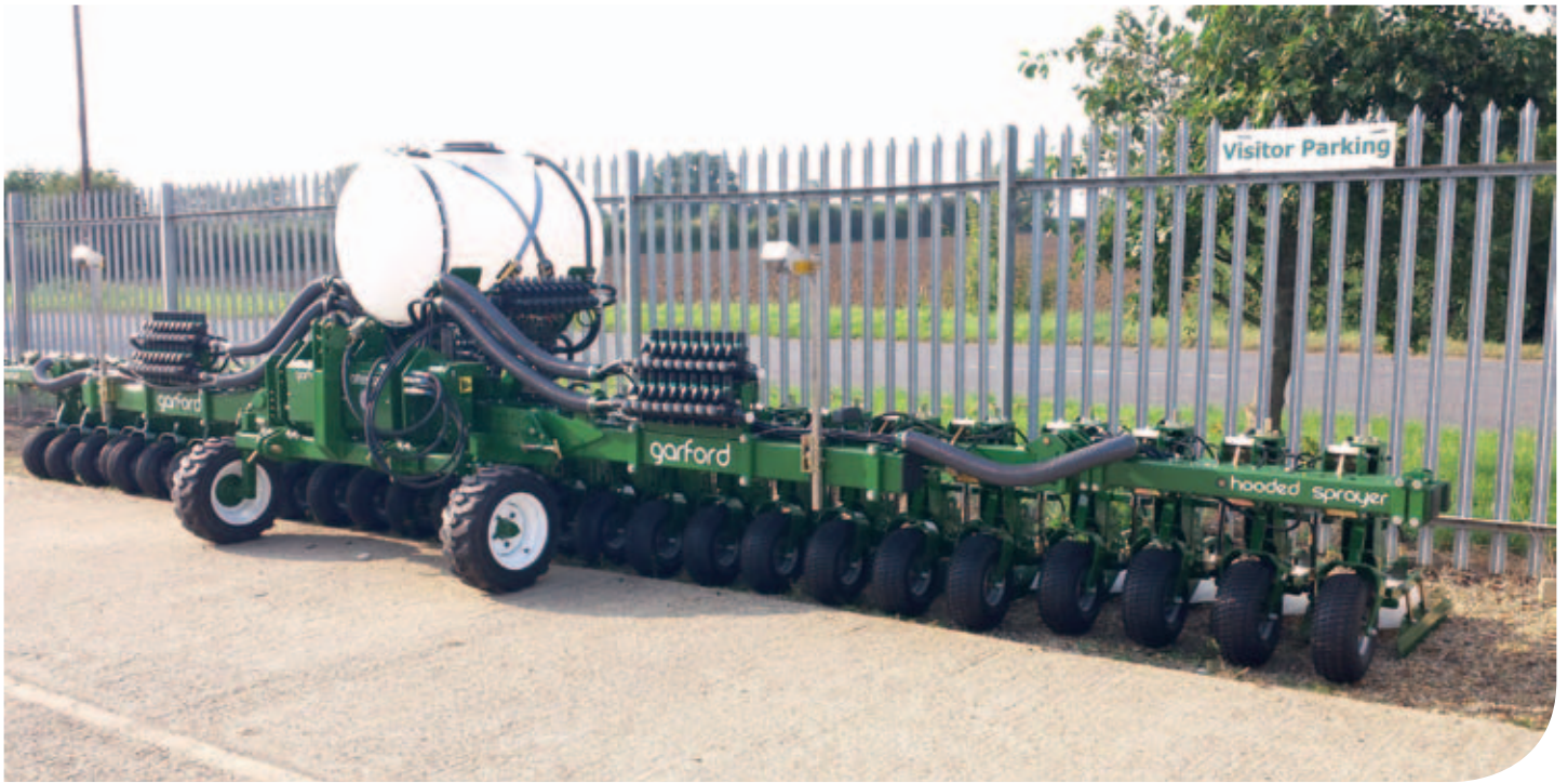
A 9mtr combination hooded sprayer and bandsprayer with Robocrop Precision Guidance and individual section control on each row!
