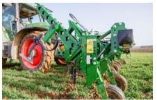
**Top-level spec**All front-mounted hoes are available with the **line raiser** function which raises the tine frames hydraulically or mechanically.
