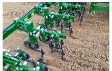
**Versatility**A front-mounted hoe adapts very easily to different applications such as the first weeding pass in maize.
