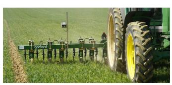
Thanks to the high-precision line and grid matching feature, the **garford** camera guidance is even reliable in windy conditions, a unique feature in the market.
